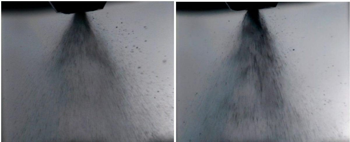
Figure 7: Water spray with atomizing air at 25 psi (left) and 35 psi (right).
