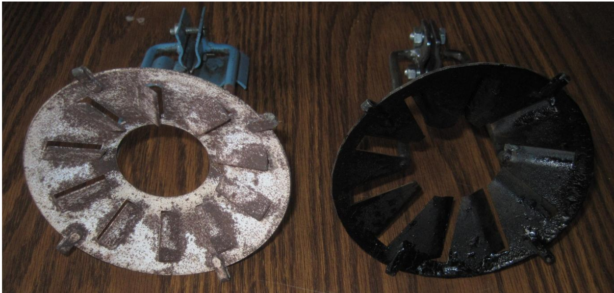
Figure 17: Original factory swirler (left) and modified custom swirler (right).
